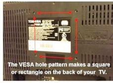
There are mounting holes on the back panel of the TV arranged in a square or rectangle pattern. The TV mount will line up and connect to these holes. You must be sure to **select a mount that has the same hole pattern as your TV**.
